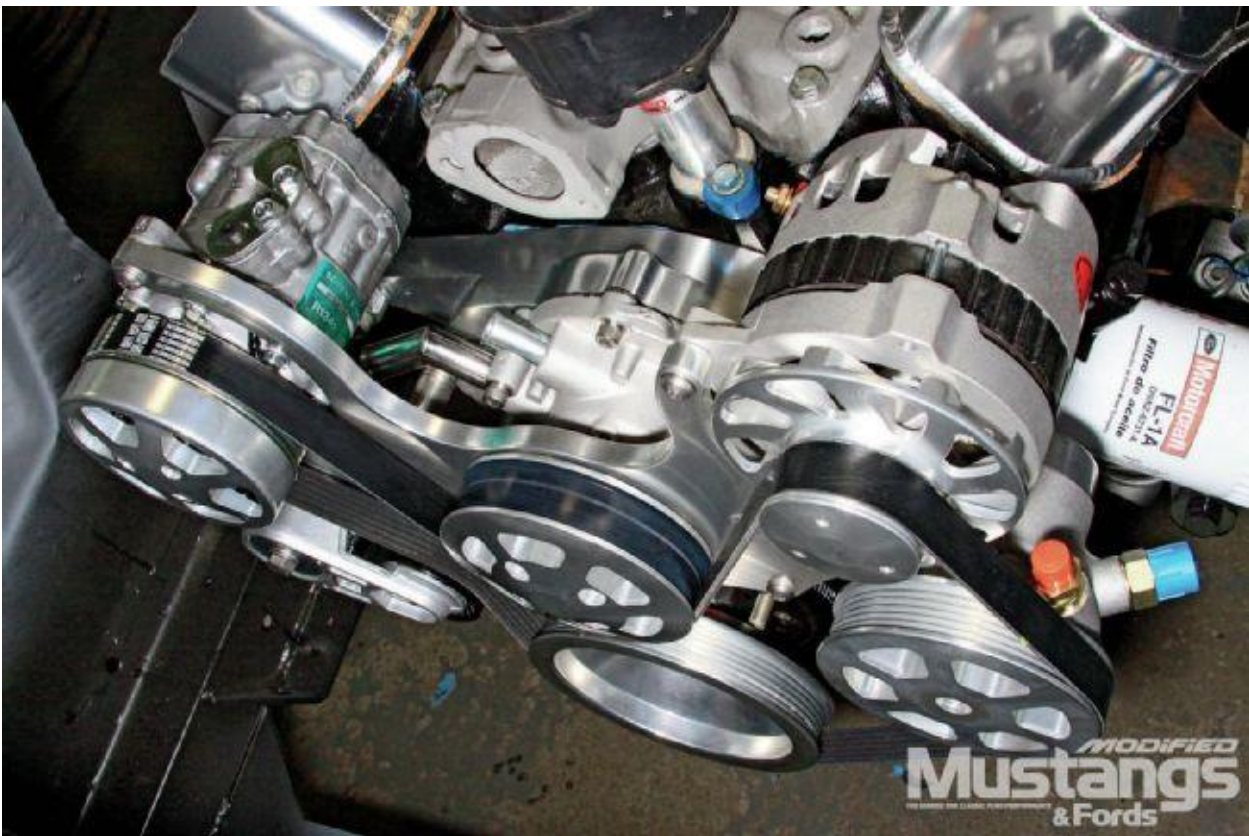
20. And there you have Eddie Motorsports' new S.Drive serpentine system. It is certainly compact, well-engineered, and it looks fantastic.
