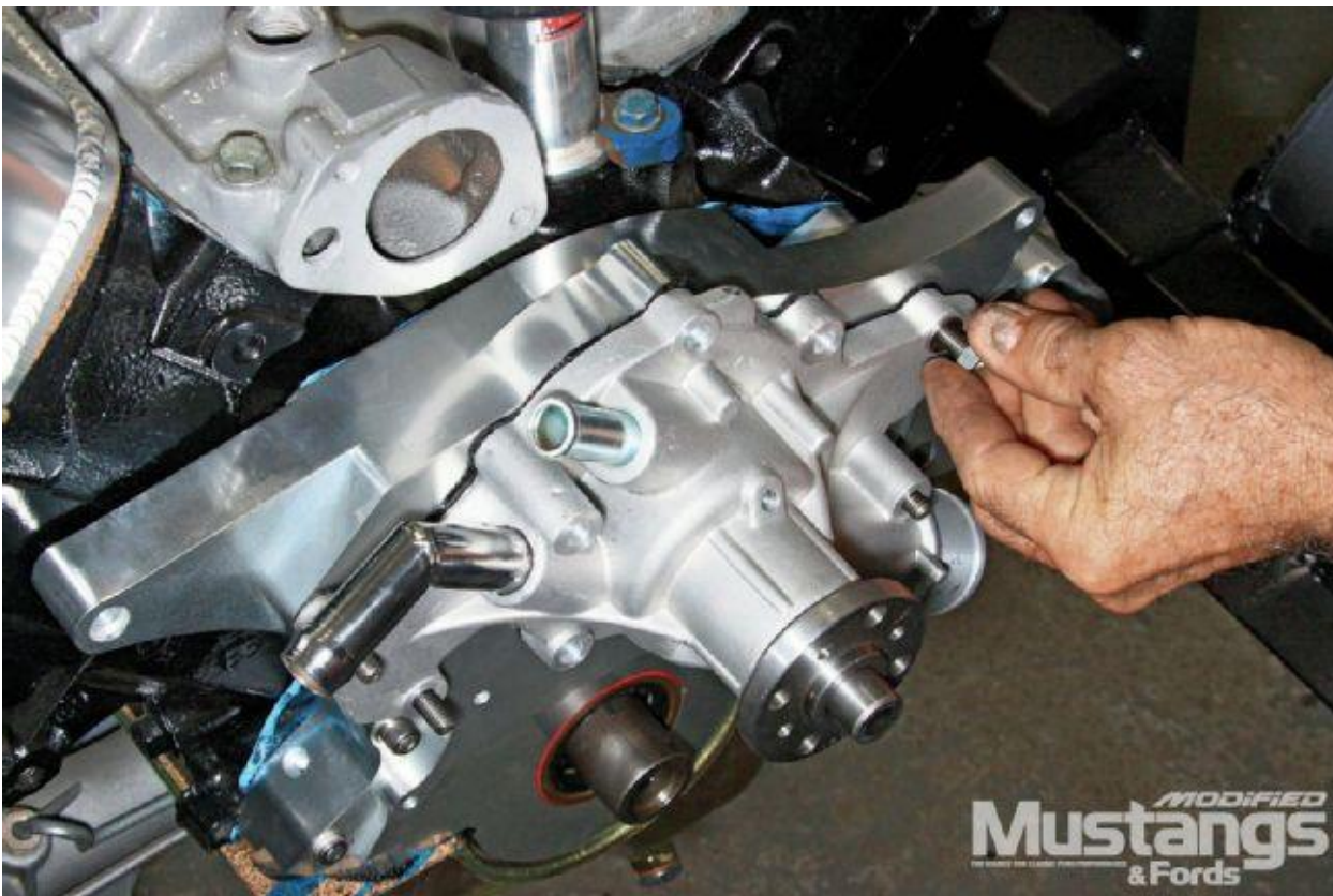
7. The water pump gasket is installed next using a thin film of Permatex Form-A-Gasket. Ford Racing's reverse-rotation water pump follows. This is also the time to install the timing pointer, which is located opposite the water pump inlet.
