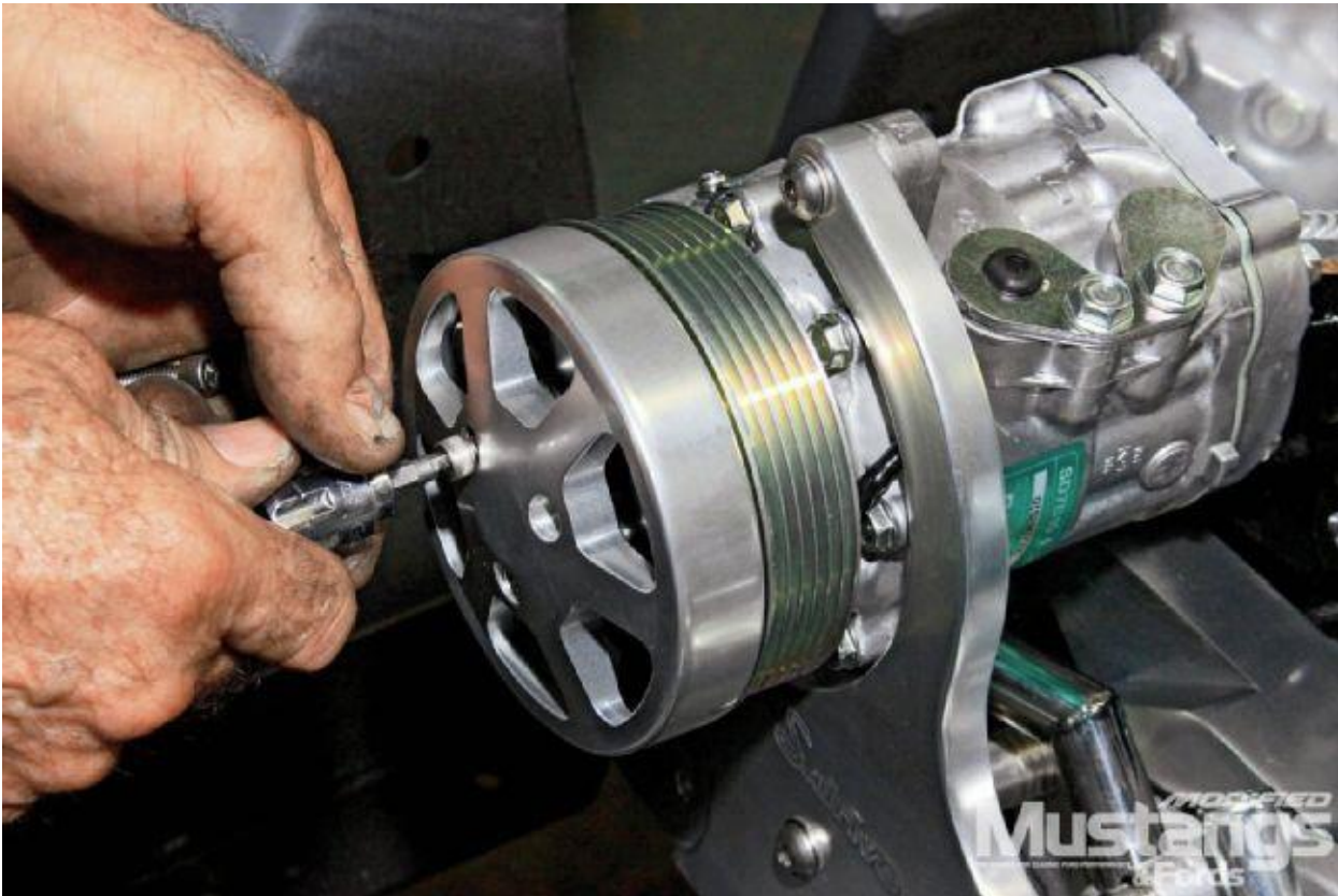
16. The compressor clutch gets this cool cover, which is bolted onto the clutch, and hides the electromagnet clutch mechanicals.
