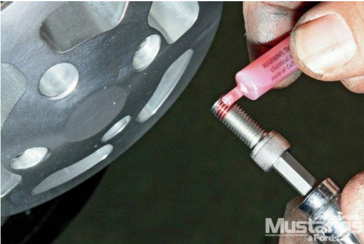
12 The water pump pulley bolts get thread locker and are torqued per the Eddie Motorsports instructions.
