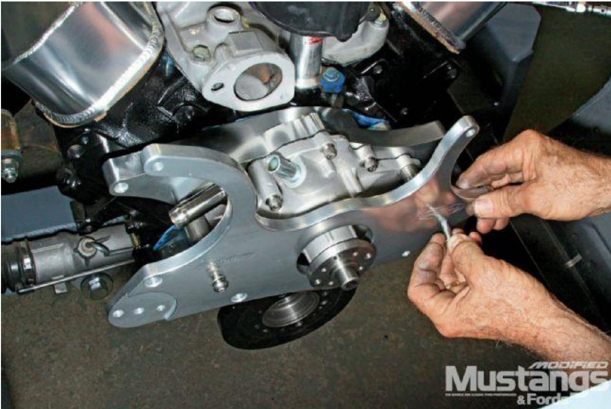
11. The accessory mounting plate/bracket is then secured to the spacer with these Allen screws.
