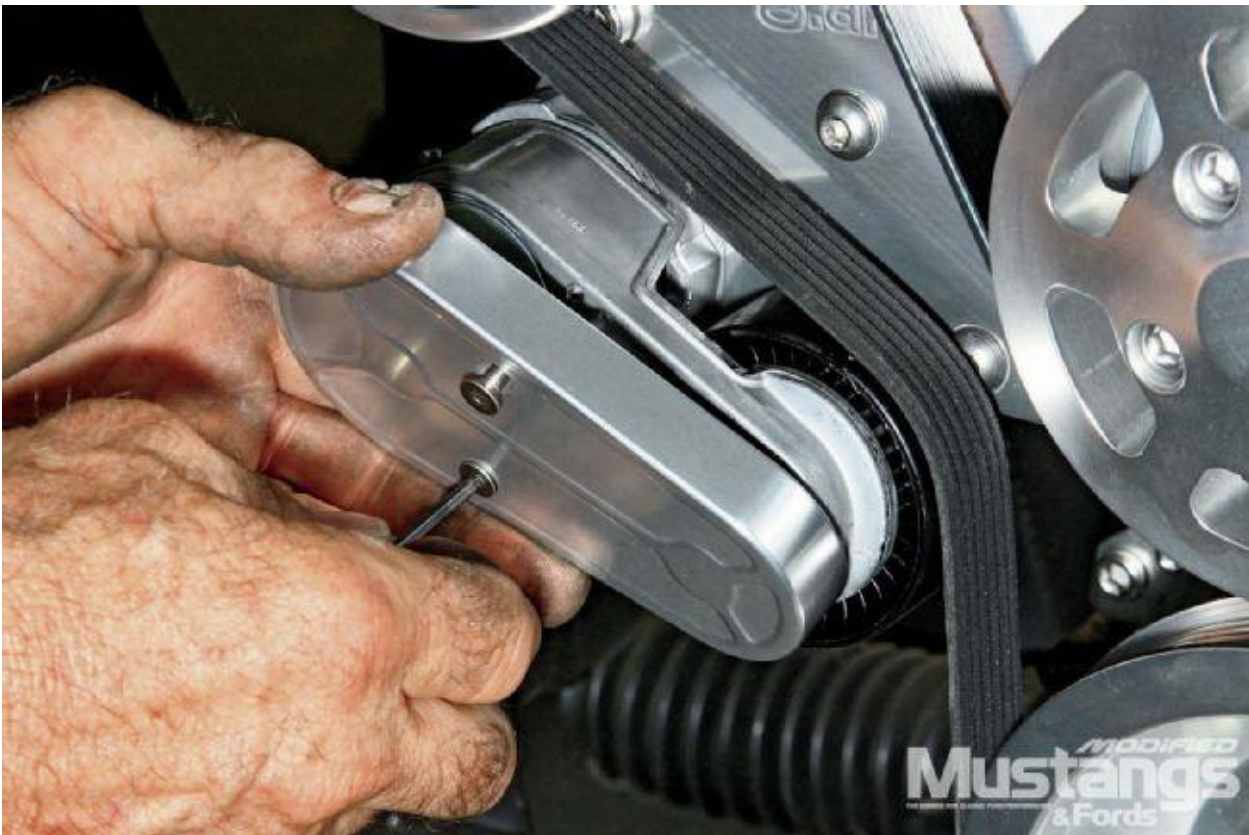
19b. The tensioner cover is installed once the belt is installed and tracking properly.
