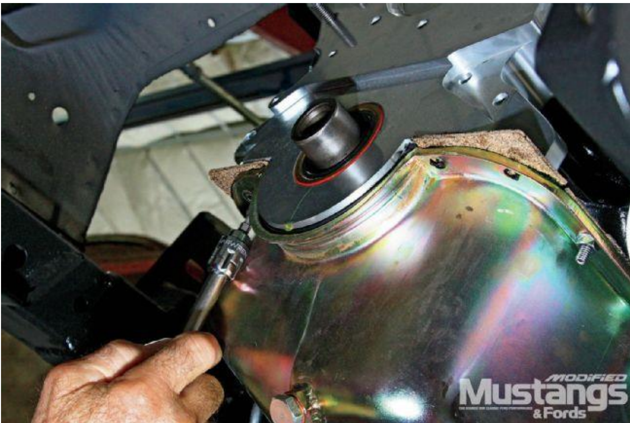
5b. The timing cover is bolted first at the oil pan for stability before the block bolts are installed. The bolt threads are coated with gasket sealer.
