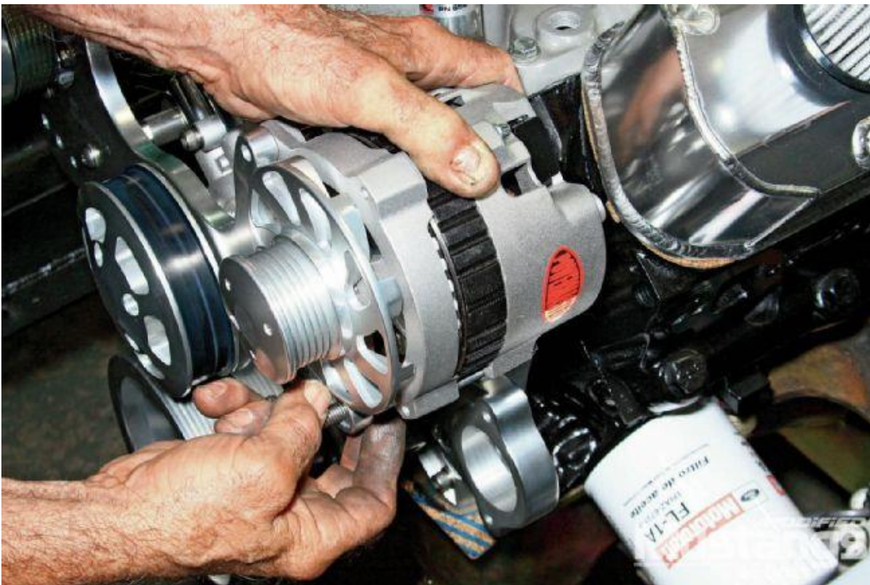
17. Powermaster's 105-amp single-wire alternator looks sharp right out of the box. Installation is easy and there's just that one heavy gauge wire to deal with.
