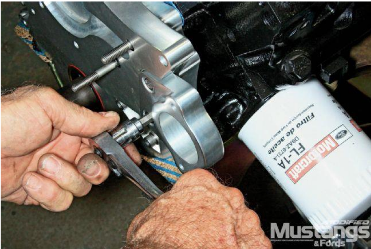
6. The Maval billet power steering pump bracket is installed next using a 16mm Allen drive.
