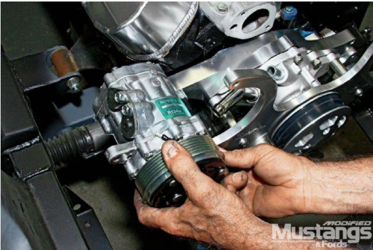
14. The Sanden air conditioning compressor is mounted next and pivots as shown. The beauty of a Sanden compressor is its rotary efficiency.
