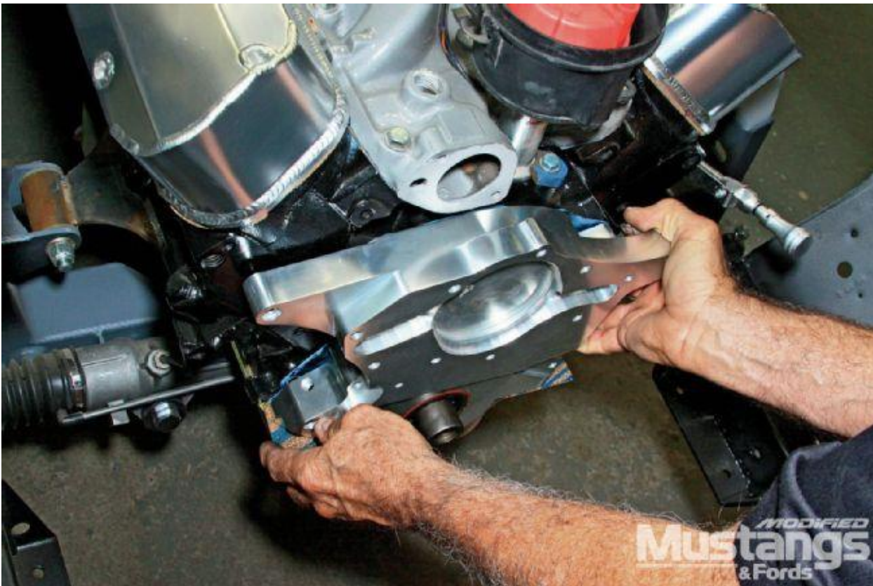
5a. The timing cover is carefully located and set in place against the block and oil pan. The pan end gasket is checked for proper installation.
