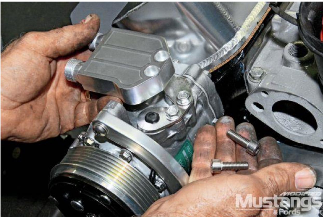
15. Included in the system is this attractive billet manifold for the Sanden compressor, which is installed last. The compressor should remain capped until you are ready to install the air conditioning lines.
