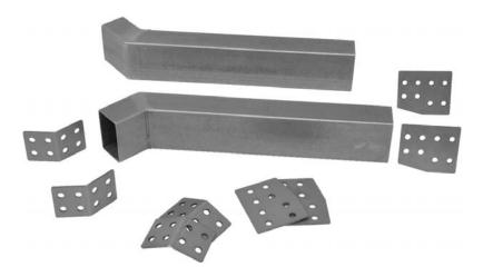
**Description:** Mini-tub frame rail insert for '64-70 Mustang. Includes rear frame rail insert sections with front and rear doubler gusset plates.
