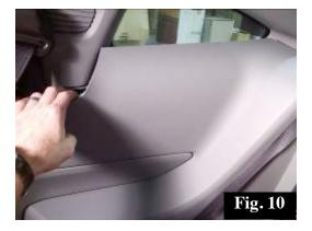
17. If the car does not have the optional Kicker 4.1 amp (part # KA-4.1-AMP) installed, signal for the subwoofer will come from the right front door speaker. Connect the supplied input adaptor (Part # RH09PIGTAIL6) to the subwoofer overlay harness two pin connector. To connect to the right front door speaker wires, first locate the wires behind the glove compartment leading to the door. Peal away a section of the electrical tape to expose the wires.
