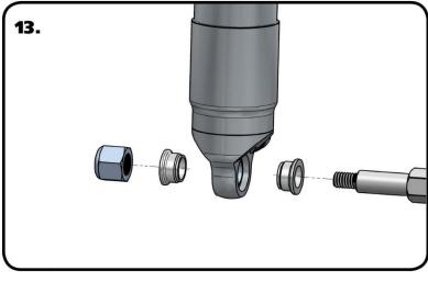
**13.** Install a 5/8" ID spacer( Small side towards shock body) onto the lower Shock Stud. Slide the bottom of the Shock onto the Stud. Install a second 5/8" ID Spacer onto the Stud(small side towards shock). You may need to jack the rearend up to Slide the Shock onto the Stud. Install the 7/16" Flatwasher and 7/16" Nylok nut. Tighten the upper and lower shock bolts.
