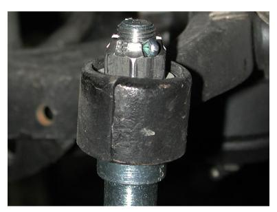
5. Install the stud with the round flange into the steering arm with the taper going into the steering arm. Torque the nuts to 35 ft lbs and tighten as needed to align cotter pin hole and install cotter pin.
