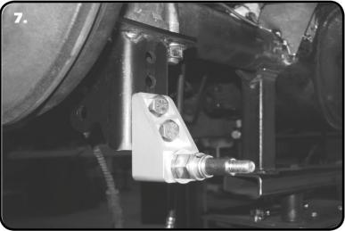
**7.** Attach the Lower Shock Mount to the Axle Mount using (1) 1/2"-20 x 1 1/4", (1) 1/2"-20 x 1 3/4" Hex Bolts, and (2) 1/2"-20 Nylok Nuts on each mount. The Shock Mount is installed in the BOTTOM 2 holes of the Axle Mount. Install a Shock Stud and 5/8" washer in each Shock Mount. Tighten the mounting hardware and the Shock Stud.
