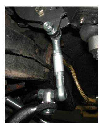
3. Attach the 90 degree end of the PosiLink to the front tab of the upper control arm using a 10mm Nylok nut and a 3/8" flat washer on each side of the tab. The nut will be towards the front of the car with the lower nut towards the frame.
