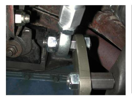
6. The studs with the short hex get installed into the draglink adapter. The short side goes into the adapter attached with the 5/8"-18 thin top lock nut, with the long side of the stud pointing forward.
