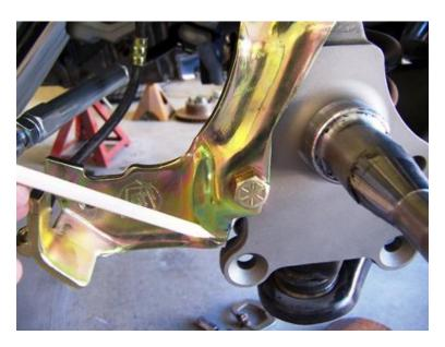
**Note:** If using a factory style stamped caliper bracket, the bracket may need to be trimmed. The dust shield may also need to be modified.
