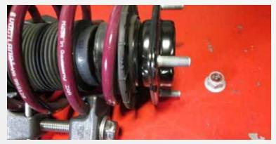
With a spring compressor, slowly depress the spring, then remove the upper strut retaining nut, then remove the upper strut mount assembly from the strut shaft.
