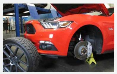
Place the front of the vehicle onto jack stands so that the wheels are off the ground.
