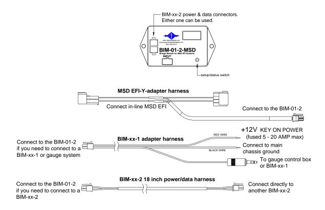
This Bus Interface Module is designed to read engine information from MSD Atomic EFI TBI kits. Atomic EFI LS is <u>not</u> compatible. This module is connected to the MSD EFI through the included Y-adapter harness. This can be plugged in line with the Atomic handheld display or the throttle body.
