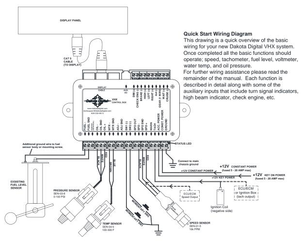
• Set up the control box to match your vehicle. The tachometer must be set to match the number of engine cylinders and the fuel gauge must be set to match your fuel sender resistance curve or the instrument system will not display correctly. The control box can read seven common fuel level sender resistance values. If your sender is not listed, the system can be programmed to a custom sender (see full manual for details).
