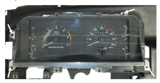
3. Connect the CAT5 cable to the back of the VHX cluster as it is installed into the dash, take care when routing the other end of this cable to the control box mounting location. Mount the VHX cluster to the dash structure using the four factory screws.
