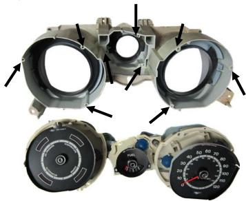
3. Mount the VHX displays into the housing using the stock hardware.
