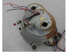
6. Using the 4 included screws provided secure the clock assembly into the housing using the light cover tab holes. It is recommended to start all 4 screws then tighten in a crisscross pattern. Place a bead of silicone around the edge of the opening that the wires pass through to keep them from chaffing.
