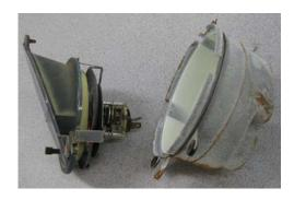
2. Remove the clock from the can. You may need to bend back the edge of the rear can for easier removal.
