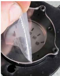
▲ The VHX gauge display for the Mustang comes completely assembled and internally wired. There's nothing you really need to do to prepare the assembly short of removing the protective plastic from the gauge lenses. We recommend doing this right before installing the bezel to prevent wayward scratches.
