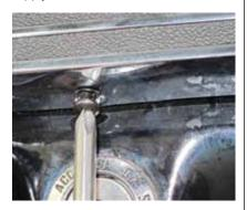
▲ The assembled display is secured to the dash with the proper black mounting screws in all six locations. The owner picked up the fasteners when he bought the new gauge bezel, which is smart thinking!
