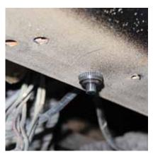
▲ The VHX system includes two momentary push buttons to control functions of the LCD screens. The '65/'66 VHX system only has one such screen so we mounted the button in an existing hole in the bottom edge of the dash; easily reachable while driving. The '67-'70 VHX system utilizes two LCD displays and you'll have to mount the second button if you wish to cycle through the second display's available readouts.
