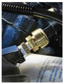
The oil pressure sender is installed in the same manner using one of the included thread adapters and the provided wiring harness. We carefully routed the wiring up to the intake and secured it to the factory wiring, routing both new sender harnesses to the firewall area.
