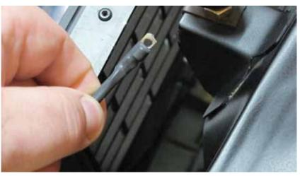
▲ Once secured, the outside temperature sensor is routed to the front of the car. The instructions state to ensure the sensor is in the car's regular airflow path going down the road. The small hole in the end of the sensor makes it easy to secure the sensor to the grille with a small tie-wrap.
