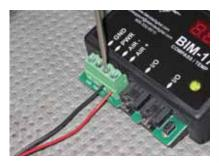
▲ Wiring of the BIM is straight forward. The temperature sensor wires are secured to their terminals and the other two terminals receive power and ground wires. The included mounting bracket makes securing the module a simple job, but note the module must be level and oriented and you have to go through the VHX setup menu to select the proper compass location.
