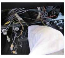
Disconnect all wiring to the gauges so that the gauge bezel can be completely removed. Most of the original wiring will not be reused except for the left and right turn indicators, the high beam indicator, the fuel gauge sender wire, one dash illumination wire, and the key switched power leading to the instrument voltage regulator. Tape or note these wire colors for later.
