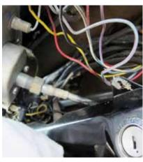
▲ Protect your steering column's paint with a thick towel and pull the gauge cluster out far enough to access the speedometer cable drive and remove it from the speedometer head by unscrewing the end of the cable.
