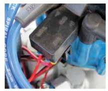
▲ Since the VHX display includes a tachometer (both in the face of the speedometer and available as a digital readout in the odometer window) a tach lead wire is required. This wire is not provided, so you'll need a sufficient length of 16-18 gauge wire to route from the coil's negative terminal (shown here as the "TACH" terminal on this HEI conversion distributor) to the dash area.
