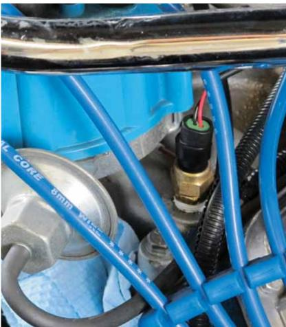
▲ Dakota Digital includes new wiring for their senders with a water sealed connection. Simply slide the connector into the sender until it locks in place. Your original single sender wire can be removed if you like, or you can discreetly tuck it into the OE harness and tape it up, which is what we did.
