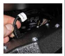
▲ The multiplex cable is simply a standard RJ-45 Cat5 network cable and just slides into place with a reassuring "click." If you want to mount the control box farther than 3 feet from the display, you can purchase general Cat5 network cables in longer lengths from your local computer supply store.
