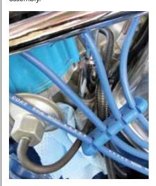
▲ The VHX system uses a set of highresolution solid-state sending units that will replace the standard senders on your engine now. Up first, we're taking care of the temperature sending unit. Simply unthread the old sender from the intake and install the supplied VHX temp sender (it's the one with a two-wire connector) and any required thread adapter, provided.
