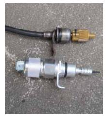
↑ The VHX system uses an electronic programmable speedometer for easy calibration no matter what driveline/tire size/gear ratio is being used. The electronic speedometer and its sensor is also how the performance calculations like 0-60 are made. As such, the stock speedometer cable will need to be removed from the car. The new speed sensor is shown here below the stock (and well-burnt) cable.
