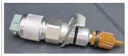
▲ The only prep for the speed sensor is to swap the speedometer cable's driven gear over. Carefully pry the retaining clip off the gear with a pick or small screwdriver and then slide the gear off of the end of the cable. Transfer the gear to the speed sensor and secure it with the original clip, as seen here.
