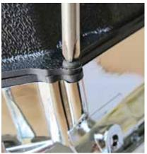
▲ Slip the gauge display into the gauge bezel and ensure the assembly is seated. Dakota Digital provides four longer mounting screws for the bottom of the new gauge assembly to mate with the gauge bezel, while four of the original mounting screws secure the top of the assembly.
