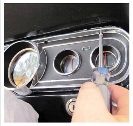
▲ The VHX gauge display bolts directly into the gauge bezel with no modifications. Simply remove the eight screws that retain the gauges to the bezel along with the lenses. If you're planning a new bezel (which this owner purchased) you simply need to remove four of the original retaining screws for the new bezel and you can set aside the original assembly for storage.
