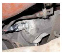
▲ The speed sensor bolts into the side of the transmission just like the old cable. The included sensor harness snaps onto the end of the sensor and then must be routed to the interior. We ended up routing it over the top of the transmission, joining up with the coolant and oil sensor wiring, and then routing all three harnesses through the old speedometer cable hole in the firewall.
